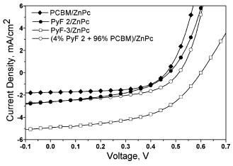
**Figure 4.** Linear I-V curves for solar cells with acceptor materials comprising PCBM, PyF-2, and 96% PCBM + 4% PyF-2 w/w mixture under  $100 \text{ mW/cm}^2 \text{ AM1.5}$  illumination.
