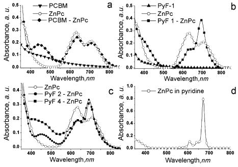
Figure 2. Absorption spectra of the ZnPc-PCBM (a) and ZnPc-PyF-1 (b) systems shown in comparison with the normalized spectra of the pristine materials. Changes in the absorption profile of ZnPc films covered with different fullerene derivatives (c); solution-state absorption spectrum of ZnPc (d).
