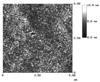
**Figure 8.** AFM image of a 4 (4% PyF-**3** + 96% PCBM)/1 MDMO-PPV blend film spin-coated on 45 nm ZnPc bottom layer.
