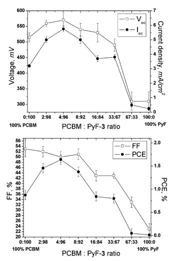
**Figure 9.** Dependence of the solar cell output parameters on the PyF/PCBM ratio used for their fabrication.
