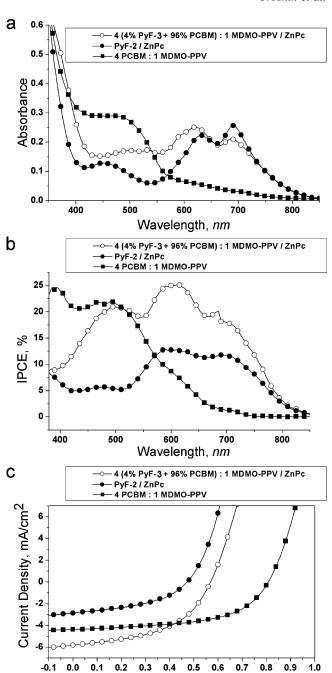
**Figure 6.** Active layer absorption (a) and IPCE (b) spectra of the bulk heterojunction PCBM/MDMO-PPV, diffusion bilayer PyF/ZnPc, and multicomponent solar cells shown together with the corresponding linear I-V curves (c).
