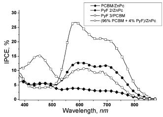
**Figure 5.** Typical IPCE spectra for solar cells made from ZnPc and different acceptor materials; PCBM is compared with PyF-2 and mixture PCBM-PyF-2 96:4 (w/w).
