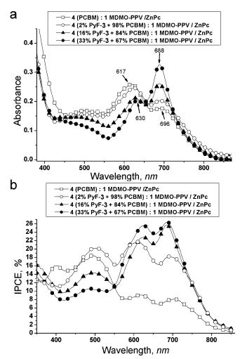
**Figure 10.** Influence of the PyF-3 loading on the active layer absorption (a) and IPCE (b) spectra of multicomponent devices.
